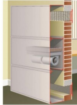
Sectional Concealed Fan Convector (would be hidden in boxing)
